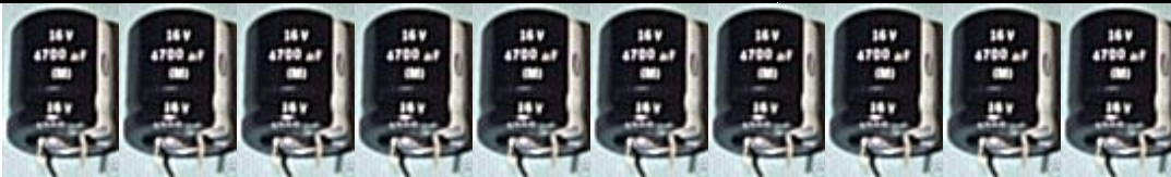
50 volt 4700uf capacitors in series.
