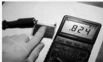
Two cells measures .824 vDC
