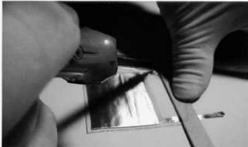
Sealing plastic with solder-iron
